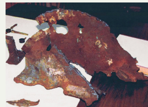
FEMA's May 2002 report documents evidence of a severe high temperature corrosion attack on the steel
